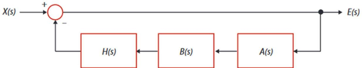
$$\begin{aligned} \frac{E(s)}{X(s)} &= \frac{1}{1 + H(s)B(s)A(s)} = \frac{1}{1 + \frac{1}{s} \cdot \frac{s+1}{s+3} \cdot \frac{K}{s^2+2s}} = \\ &= \frac{1}{1 + \frac{1}{s} \cdot \frac{s+1}{s+3} \cdot \frac{K}{s(s+2)}} = \frac{1}{\frac{s^2(s+3)(s+2) + K(s+1)}{s^2(s+3)(s+2)}} = \\ &= \frac{s^2(s+3)(s+2)}{s^2(s+3)(s+2) + K(s+1)} \end{aligned}$$
